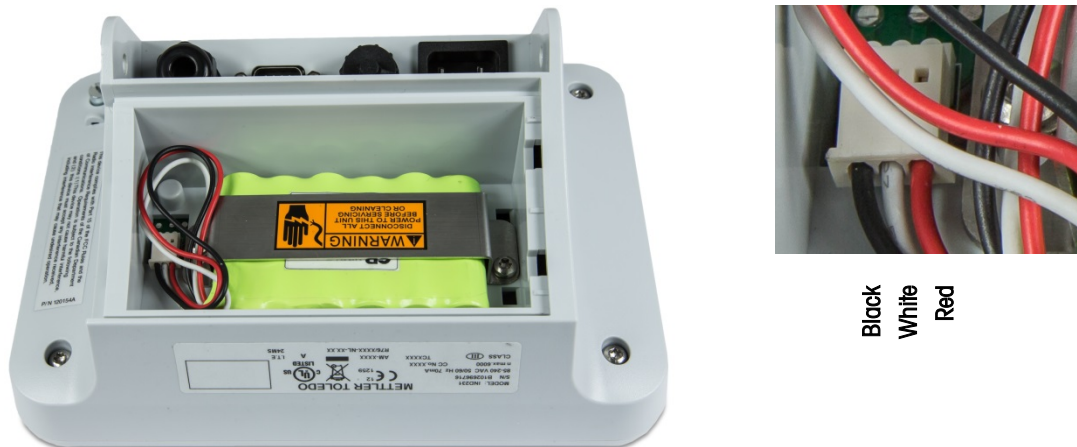
Figure 2-21: NiMH Battery Installed in IND231
