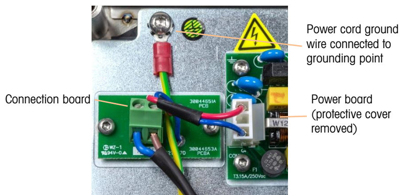
Figure 2-18: IND236 AC Power Connection Board and Grounding
