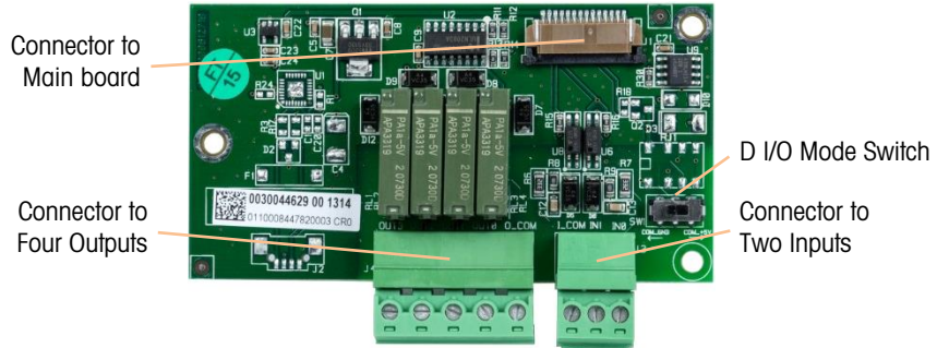
Figure 2-40: Discrete I/O Option Board
